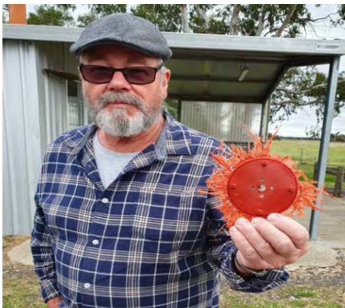
Unusual shredding pattern of the rear of the spinner backing plate, no evidence of the number of revolutions required to get this effect. Modern art.
