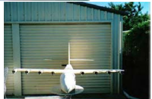
Trial fitting of components with wings sheeted and 8 motor mounts fitted
