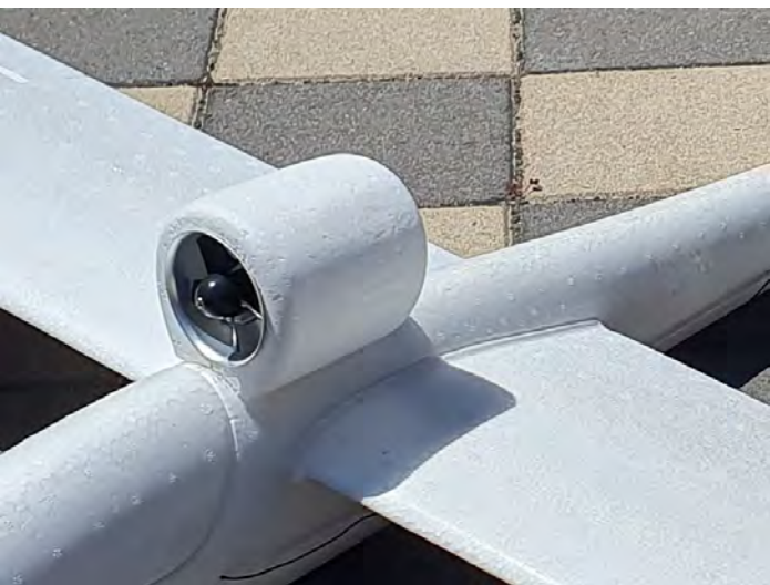
The 50mm EDF 6 blade fan power unit moulded in foam fitted to the top of the glider.
