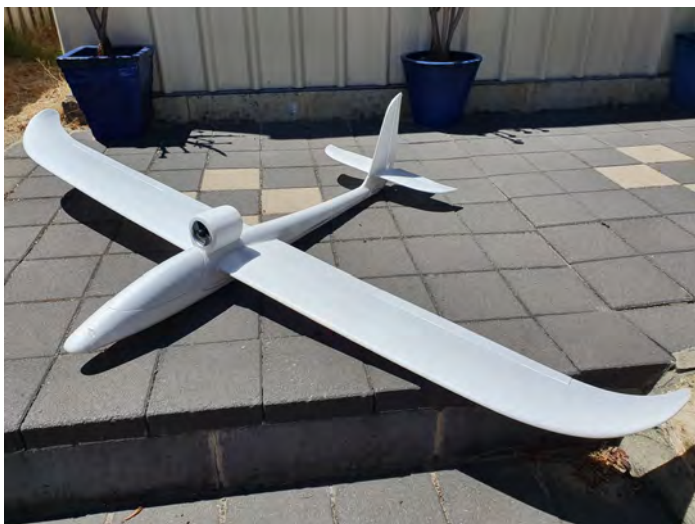
The 50mm EDF 6 blade fan power unit moulded in foam fitted to the top of the glider.
