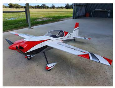
Motor being used is a Dualsky GA 6000 (180 kv) swinging a 24 x 13 Falcon Carbon Fibre prop.
