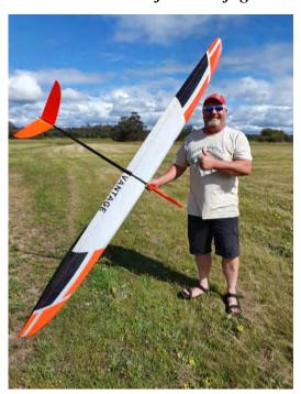
A Vantage model that flew very well after a few hand launches to sort out the trimming prior to putting it onto the winch line. Eddie indicated the most nervous moments of a new model launch is when you let the model go on the winch and quickly bring you hand down to find the control stick on the radio whilst still focusing on a very rapid launch
