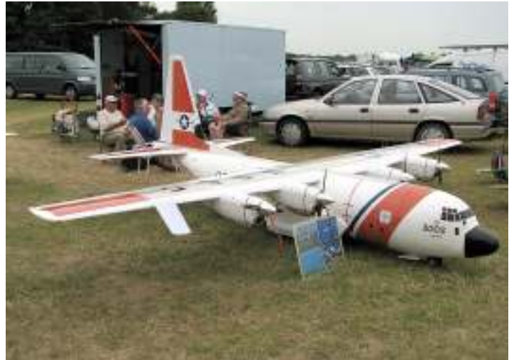
Simple set up option for getting into jet power. The plane is a test/tutor plane for PST jets. This jet gives about 7kg thrust.
