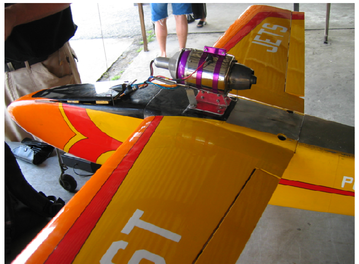
Simple set up option for getting into jet power. The plane is a test/tutor plane for PST jets. This jet gives about 7kg thrust.
