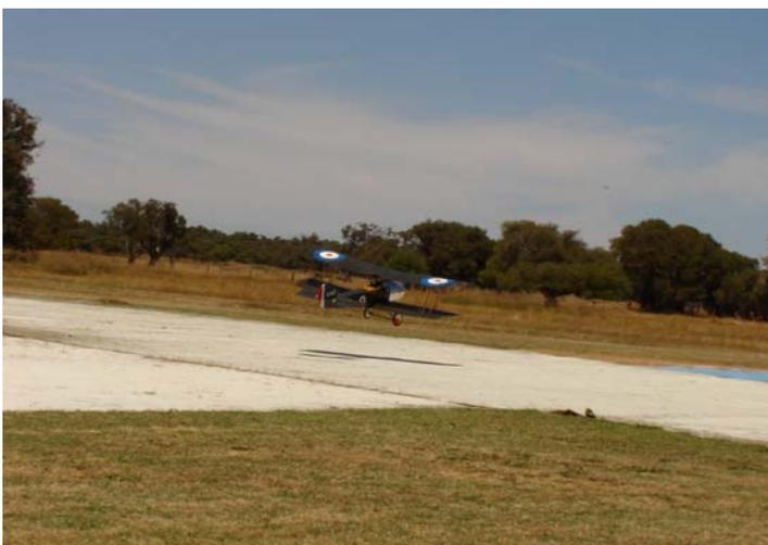
*This was the second take off, a strong cross wind caught the plane as it lifted off, full right ailerons here to correct and full throttle which pulled the plane up from any danger.*
