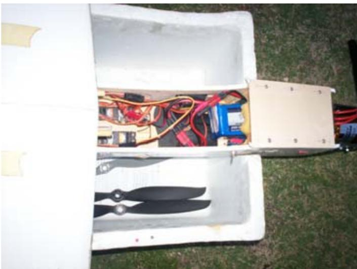
The equipment used is a Turnigy 4260-500 motor and 70A ESC with 2x 6S 3000mAh batteries in parallel (20-30C). All up cost was only around \$150 from Hobby City. I have run several props with the following results -
